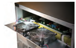
Redundant fan design enhances system reliability*
