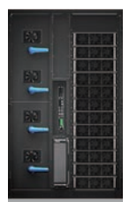
DPH 500-600K model is highly integrated with four built-in switches
